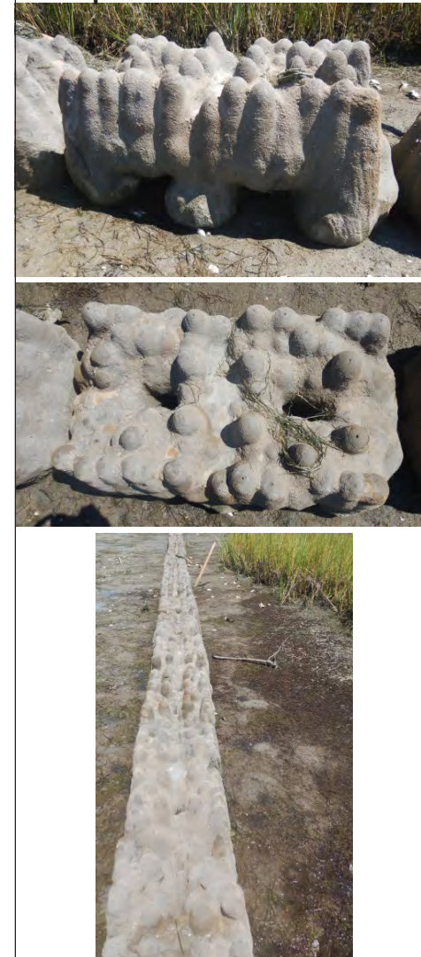
Example of a small concrete oyster structure and placement at a site.
